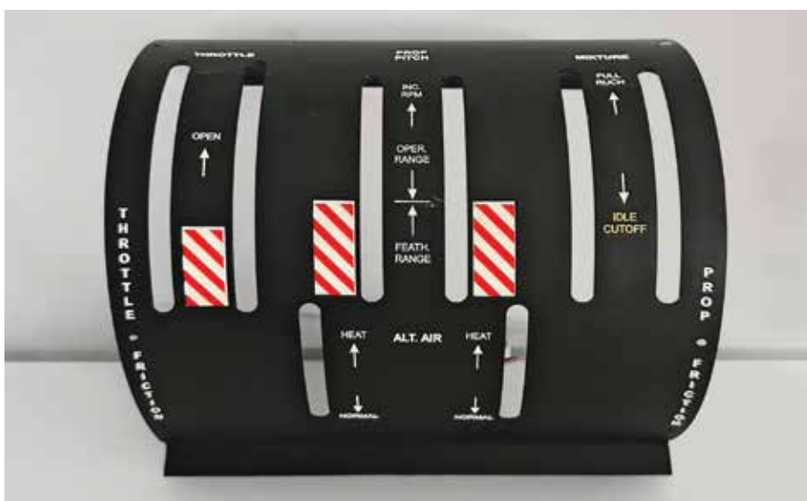
Superior Aircraft Components' Electro Luminescent Super Thin (ELST) EL panel.
