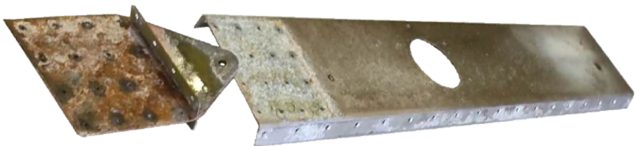
CORRODED SPAR AND ATTACH FITTING (REMOVED FROM AIRCRAFT)
